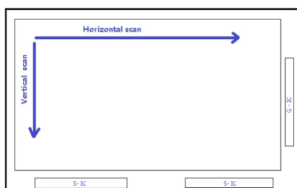
Fig. 1 Normal scan (Pin24, Reverse = Low or NC)
