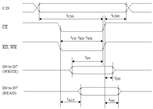
Test Conditions(Unless Otherwise Noted, VdD =  $5.0\pm10\%$ , Vss = 0V, Ta=-20 to  $75^{\circ}$ C)
