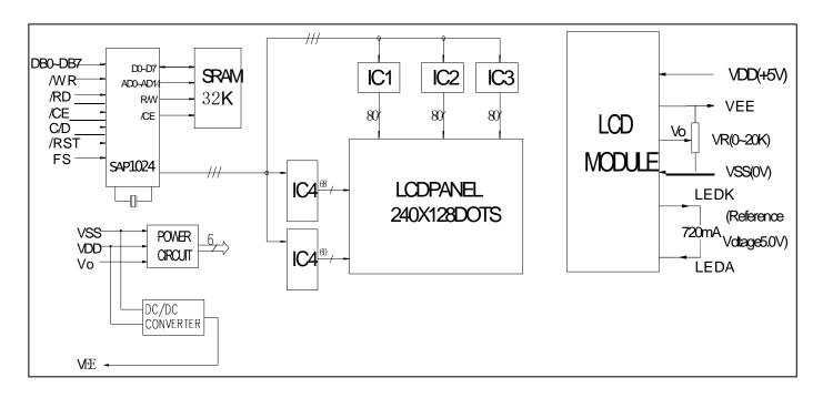
Figure 1. Block diagram
