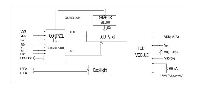
Figure 1. Block diagram
