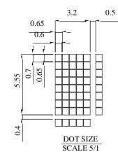
The non-specified tolerance of dimension is  $\theta$ .3mm.
