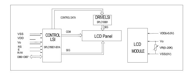
Figure 1. Block Diagram
