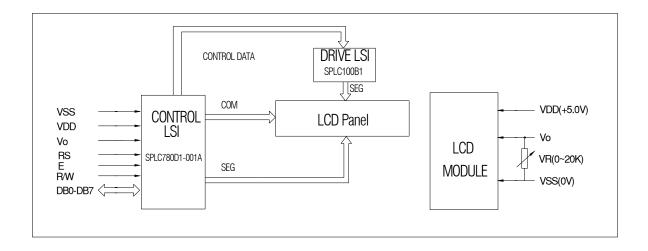
Figure 1. Block Diagram
