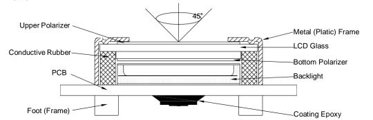
2. View Angle: with in 45° around perpendicular line.
